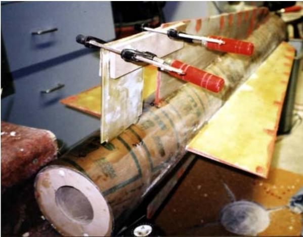
Body tube was 6" Sono Tube with several layers of 6 oz cloth. Slots were cut out to accommodate the fins. The upper centering ring was triple 1/4" airply. The shock cord mount was a 5-inch square post mount with large washers to spread the load around during deployment. The motor tube with centering rings glued on was slide into place then each ring on both side where glued to the tube wall. Note that Sono tube has a wax layer
