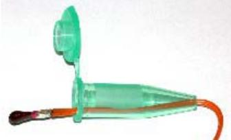
It just so happens that these graduated micro centrifuge tubes hold 2ml of fluid. So in the lab I carefully measured out 1.0 grams of FFF Black Powder (BP) and it was very close to the 1ml mark on the tube. I did the same for 1.5 grams and 2.0 grams, they also were very close to the corresponding graduated marks on the tube.
