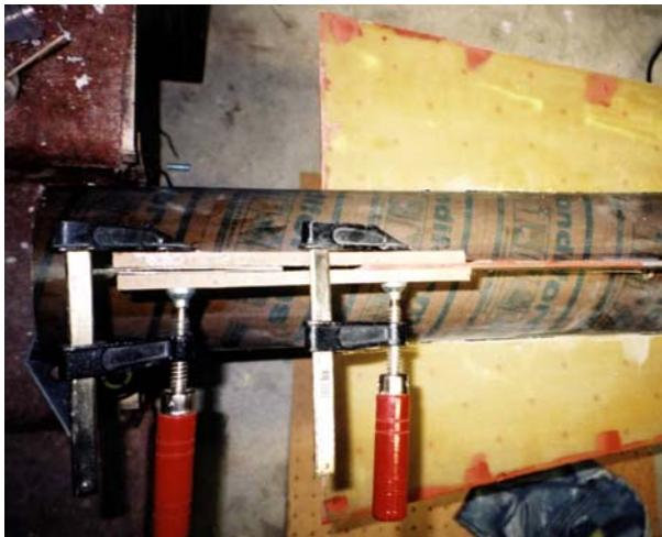
Fin alignment was first done through careful measuring and cutting of the fin slots to ensure it was parallel to the tube. Secondly, I created a jig from 1/4" hard board that fit closely on the
