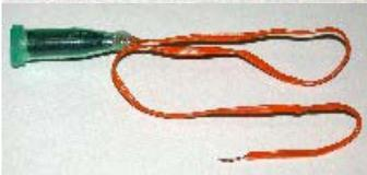
I wrap the bottom end of the tube with tape to prevent any of the BP from spilling out. I pour in my BP, pack the top with cellulose wadding, snap the lid on and I have a ejection charge made up in a matter of minutes.
